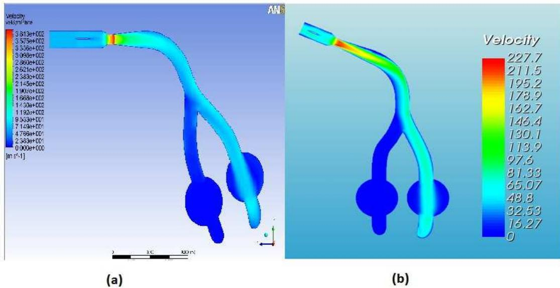
Fig. 5 Velocity field: Fluent (a) Vs KARALIT (b) results.
