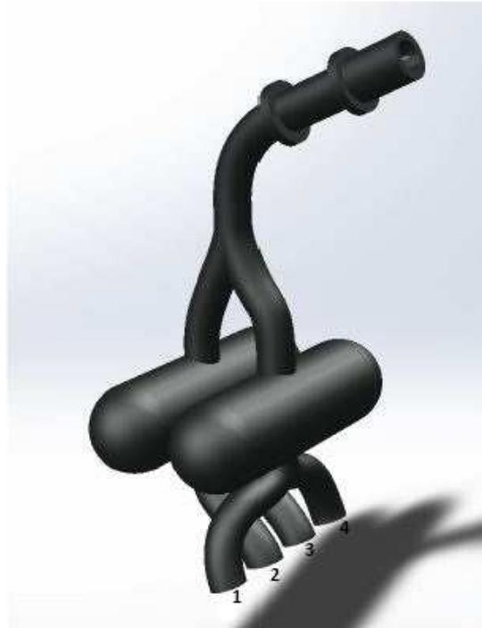
Fig. 1 Formula SAE 2013 single-seater intake manifold.
