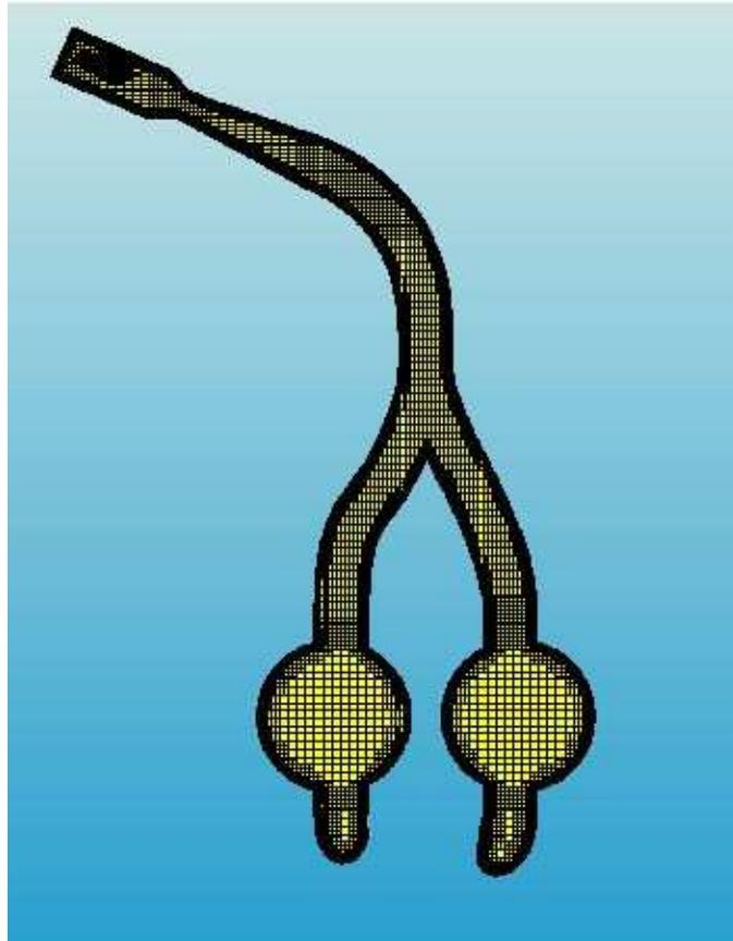
Fig. 2 The grid on the plane of symmetry.
