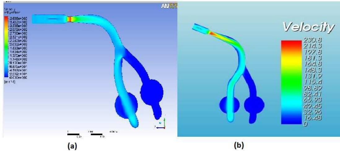
Fig. 4 Velocity field: Fluent (a) Vs KARALIT (b) results.
