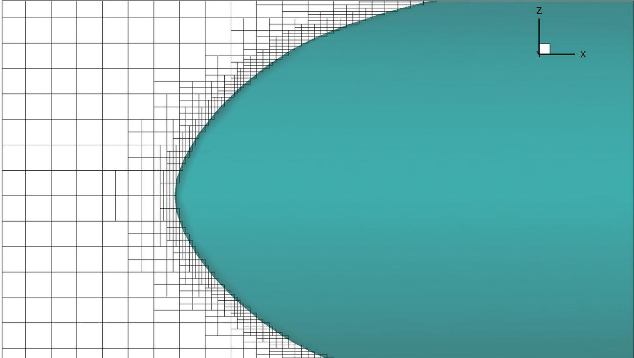
Only the cells whose center lies in the fluid domain region are solved by the equations. The Boundary conditions are applied at additional nodes located on the surface, and not on grid nodes. This is what the IB mathematical technique is all about.
