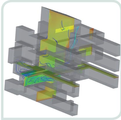
*Internal Temperature Distribution and 3D flow field within the University Building.*
