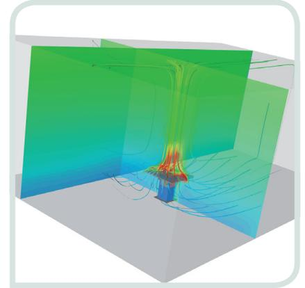
*Example of a room heating from a bioethanol fireplace. Clearly shown the nice thermal plume derived by the use of the buoyancy model in KARALIT CFD (Courtesy of Brantabee).*
