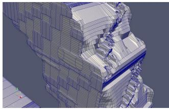
Curved pipe with a square cross section: Cut-Cell
