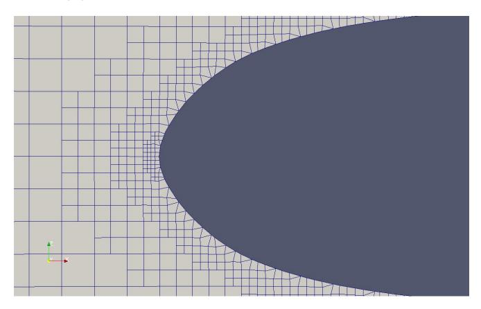
The following figure shows how a cut-cell method re-shapes the cells near the body:
