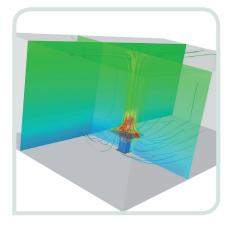
Example of a room heating from a bioethanol fireplace. Clearly shown the nice thermal plume derived by the use of the buoyancy model in KARALIT CFD (Courtesy of Brantabee).
