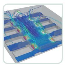
Internal Temperature Distribution and 3D flow field in a car park with cars.
