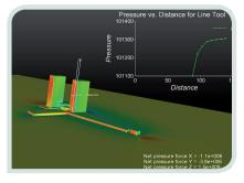
An example of how KARALIT CFD can be also useful to determine the pressure and forces distribution over a building facade, in order to give to the civil engineer or architect the right informations for a subsequent structural analysis.
