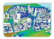
Velocity distribution at a specified height from ground, to assess the compliance of the design in evaluating any possible discomfort of the pedestrian around specific urban areas.
