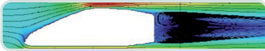
Flow streamlines and contours of U-velocity, depicting flow separation at the rear of the model on a symmetry plane.
